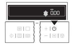
2. Using the +/— button, set the desired countdown (max. 99.00 minutes).
